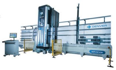
**<sup>\*</sup>D-Shaping** is the first device that allows you to work shaped glass sheets on the vertical CNC.
